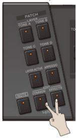
3. To select the step to record, hold down the desired [1]–[16] button and press the [NOTE] button.
